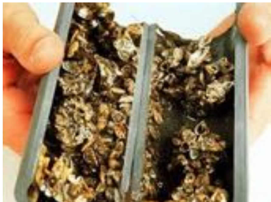
Cross section of a pipe clogged with zebra mussels
