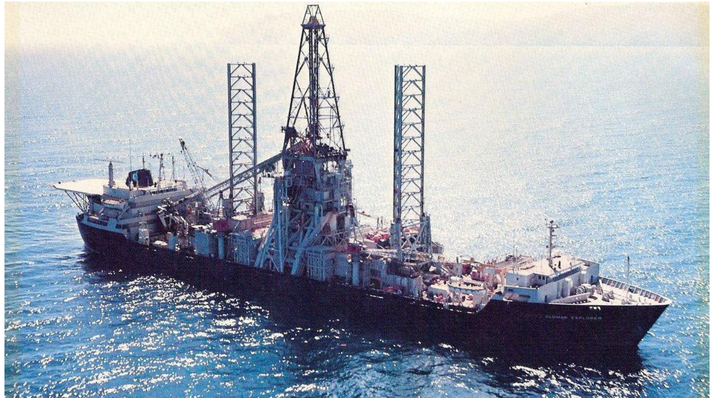
Glomar Explorer 1974 (nodules) (cover for CIA recovery of Soviet K-129 nuclear submarine, 5000 m)
