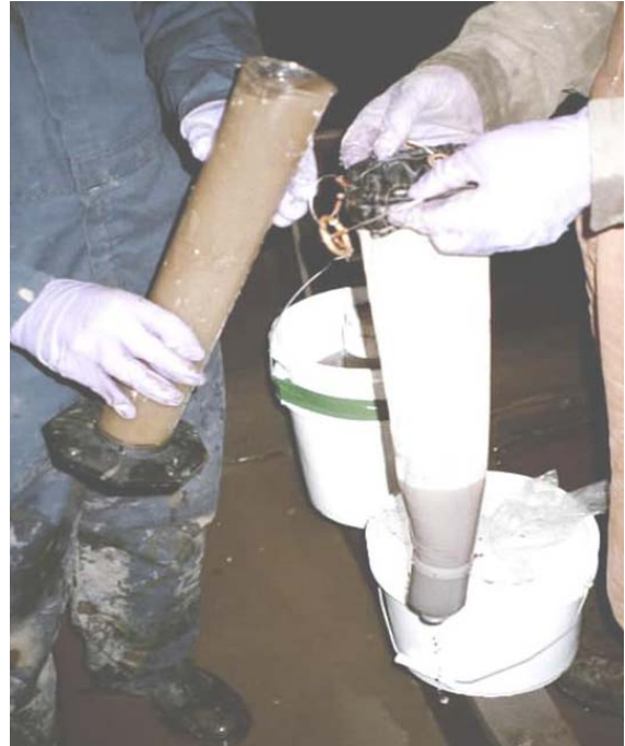
Figure 2. Ballast sampling includes collection of water and sediment samples to examine the diverse collection of phytoplankton and other invertebrate fauna (Great Lakes NOBOB Assessment Program, NOAA).
